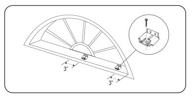
**Shades stacking on the right**, mount one installation bracket approximately 3" from the right side of the opening and the other bracket 3" to the right of the center of the window opening.
