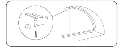
(1) Mount the top clip at the top center of the arch opening.
