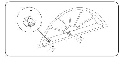
**Shades stacking on the left**, mount one installation bracket approximately 3" from the left side of the opening and the other bracket 3" to the left of the center of the window opening.
