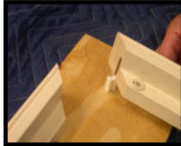
Set Hoffman Key round side up and push top frame down onto the Hoffman Key
