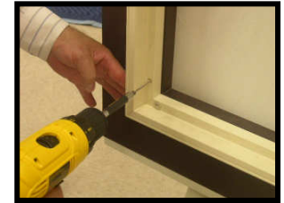
Only secure one screw into the bottom left frame.
