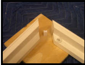
Set Hoffman Key round side up and push top frame down onto the Hoffman Key
