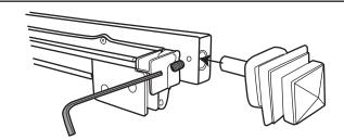
5. Clip traversing track onto the brackets on the wall; make sure track is securely in brackets.
