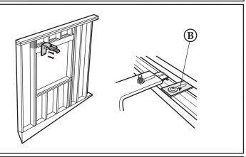
3. Adjust projection of bracket clip by loosening the screw nut (C). Adjust bracket projection as needed. Retighten the screw nut to hold the clip in desired position.
