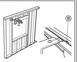
3. Adjust projection of bracket clip by loosening the screw nut (C). Adjust bracket projection as needed. Retighten the screw nut to hold the clip in desired position.
