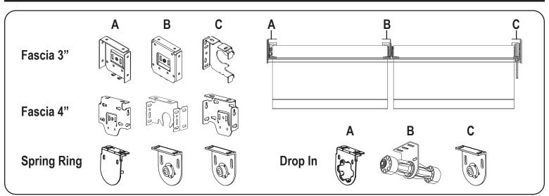
On Fascia 3 and 4" System, the edges brackets (A and C) are the same. On the Spring Ring and Drop in systems, the "A" bracket should be placed on the edge at the motor side. The "C" brackets should be installed at the idle edge. The Intermediate Brackets (B) should be located between shades.
