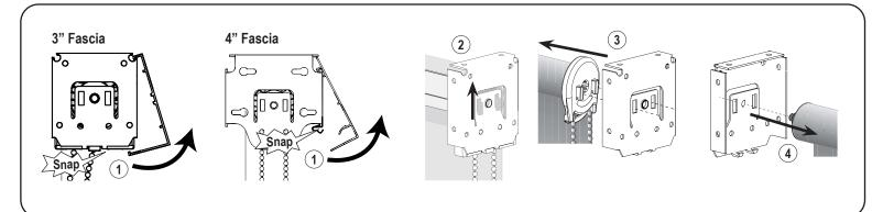
First, rotate upward to disengage the fascia. Then, gently pull up the control unit (Clutch, Motor or Spring) until the hooks touch the top part of the bracket slot. Pull the shade towards the spring loaded pin end until the hooks are complete out of the bracket slots. Finally, remove the spring loaded pin end from the idler bracket.
