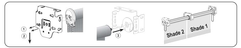
Install the final regular bracket aligned and leveled with the others. Place the spring loaded pin end into the round hole of the intermediate bracket. Keeping the pin end secure in its bracket, insert the hooks on the clutch straight into the two slots in the bracket. Once the two hooks are through the slots, gently pull downward on the side with two hooks until the two hooks have locked securely to the bracket.
