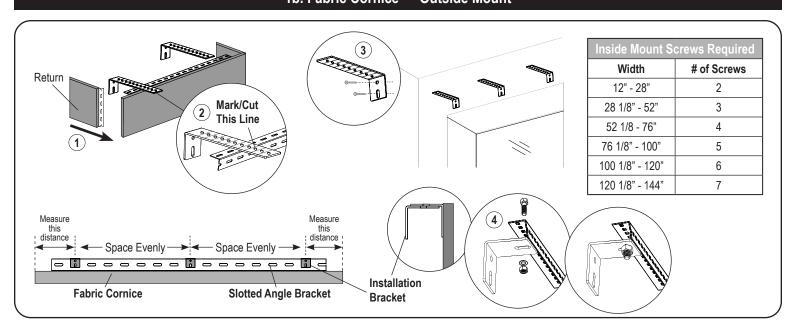
First, attach the returns to the valance and check the angle on each return. Then, fasten short screws into the valance. Repeat for opposite return. If ordered custom returns under **Fabric Cornice Only (without shade)**, place the 8" bracket on top of the slotted angle next to the return. With the back of the bracket flush with the back edge of the return, mark the cut mark just past the screw hole that lines up with the slotted angle. Then cut the bracket at the mark.
