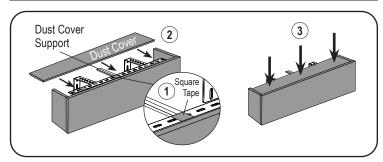
First, snap the dust cover support onto the slotted angle. Then, remove adhesive backing from square tapes and place the square tapes on slotted angle and brackets. Press the dust cover in place to secure the adhesive.
