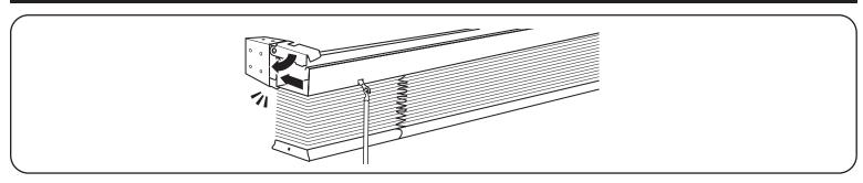
Slide blind into bracket and snap door closed. Use both hands on the bottom rail to lift or lower blind. Rotate wand to tilt slats. Blind slats should be tilted open prior to lifting and lowering.
