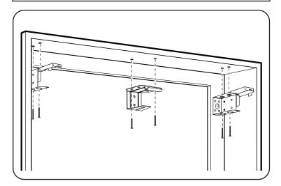
Drill pilot holes and install brackets using screws provided.
