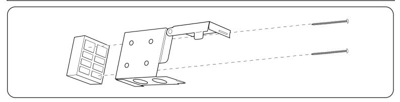
Spacer blocks provide an extra 3/8" clearance behind blind to clear obstructions like window moldings. Attach blocks to the end of each bracket. Use longer screws included with spacer block kit.
