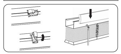
Evenly space valance clips on backside of the valance. For Inside Mount, attach valance before blind installation. For Outside Mount, attach valance after blind installation.
