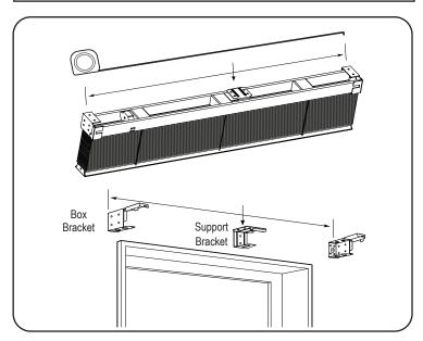
Place box brackets on headrail. Evenly space support brackets between box brackets, away from ladder cords. Using a tape measure, measure bracket locations. Mark bracket positions.
