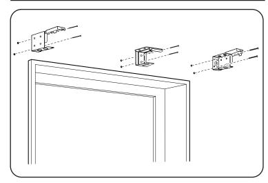
Drill pilot holes and install brackets using screws provided. Wall anchors may be required for secure attachment (not included).
