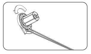
Add the replacement bead chain by first feeding the chain under the guard on the bottom of the clutch. Then, begin threading the new chain around the gear on the clutch by pulling and turning the gear until the chain is fully engaged.
