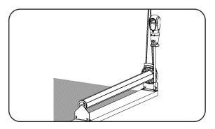
Use a screwdriver to remove the bracket anchoring the clutch to the headrail.
