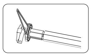
Insert the clutch into the tube with the bottom of the clutch positioned straight down. Align the bracket and clutch onto the headrail then use the screws to secure the bracket.
