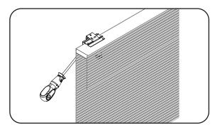
Lower the shade all the way down, then detach it from the installation brackets.
