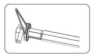
Detach the bracket from the clutch, then remove the clutch from the tube.
