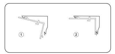
Re-install the shade by snapping the headrail connector into the installed mounting bracket.
