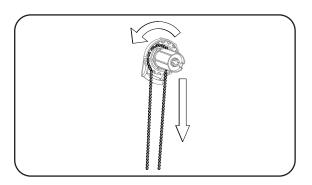
Remove the bead chain by unthreading the chain from the gear of the clutch. Gently pull the chain away from the clutch while rotating the gear until the chain is completely released.
