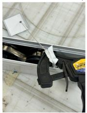
We put some duct tape on our clamp as it is old and the rubber clamp pieces are a bit hard
