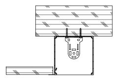
Do not mount shade brackets to endplates. Install brackets into blocking or building material directly.
