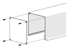
Install endplates using #6 flathead screw.
