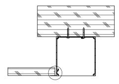
Always make sure that mounting screws are securely tightened into the blocking or material that the Pocket is being mounted to.
