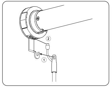
On Banded Shades, Roller Shades and Sheer Shadings, with the wand control buttons facing you, attach the top of the wand on the metal hook support (1) on the motor control side, then connect the cable into the motor head (2). **Note:** On Sheer Shadings ordered with Powerwand on the right side, the cable may be wrapped around the hook. This is normal. You may unwrap, if you desire, as this does not affect functionality. You still need to connect the cable into the motor head.
