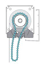
SL10 & SL15: Attach Chain Diverter Cover
