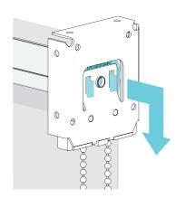
Align the chain in the diverter (SAME POSITION FOR ALL CLUTCHES)
