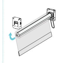
Ensure Clutch Hooks engage Bracket
