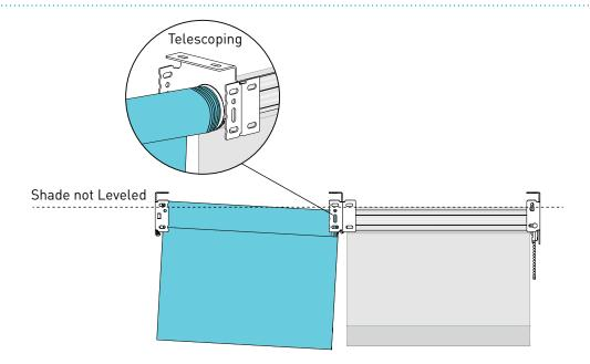
Adjustment of the bracket is needed when the window has not been framed correctly or the structure settles. This can lead to uneven light gaps on the side or telescoping.
