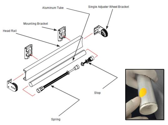
**Note:** Position of spring and stop depends on type of Roman shade you're making. When assembling your shade, use a sticker or similar to mark spring side for later reference.
