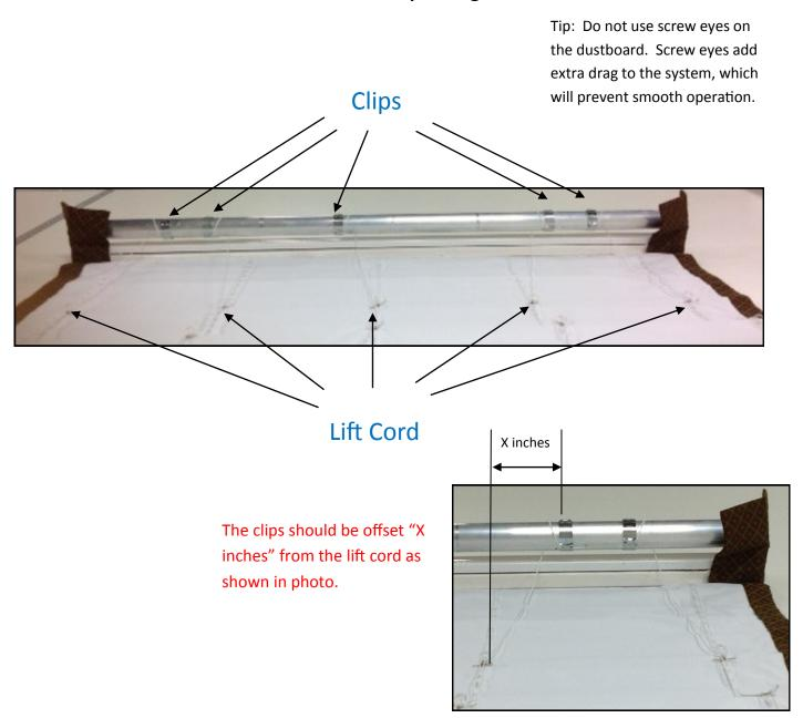
15. Clips should be spaced evenly with "X" inches between the lift cord on the shade and the clip on the roller tube. "X" equals 1" for shades up to 30" in length, 2" for shades between 30" and 60", and 3" for shades over 60" in length. Shade should be fully extended during attachment. Cord should come between tube and headrail and over top of tube for attachment. Center cord may go either to the right or left.
