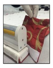
19. Completed shade. Visually check to make sure that the spring marker is on the correct side of the shade for the model that you are making. (See page 3)
