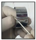
14. Attach cord clips to tube with cord knot on side nearest vertical cord lift line. (see next page for clip alignment)
